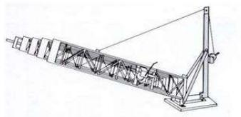
Standard model tower raising fixture for TMM, TX and HDX Series towers. Both TRX-80 and 80HD are designed to be easily mounted on your towers' hinged T-base for quick and safe one man installation or antenna servicing.
